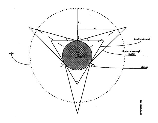
$R_c$  = Mean radius of the Earth (6378 km)  $R_o$  = Altitude of orbit (variable)  $(R_e+R_o)$  = Radius of orbit (dashed lines) (km)  $2\theta$  = Angle intercepted by ( $\theta_e$  = minimum LOS elevation angle) LOS (out of total orbit)  $x_1$  is derived in Appendix A
