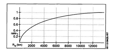
Visibility is 100 percent at  $R_0 = (1.88)R_e$ , which is 1.88 times as far as the 0 degree (local horizontal) two-dimensional model (see comparison). \*\*Note that visibilities can exceed unity (i.e., more than 100-percent visibility) because of overlap of the three stations.
