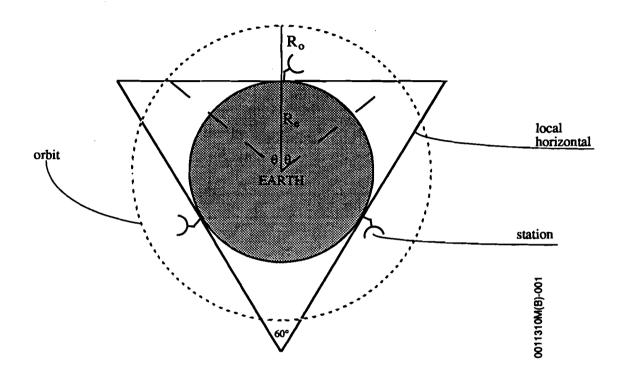
$R_e$  = Mean radius of the Earth (6378 km)  $R_o$  = Altitude of orbit (variable) (km)  $(R_e + R_o)$  = Radius of orbit (dashed lines) (km)  $2\theta$  = Angle intercepted by local horizontal {out of total orbit}
