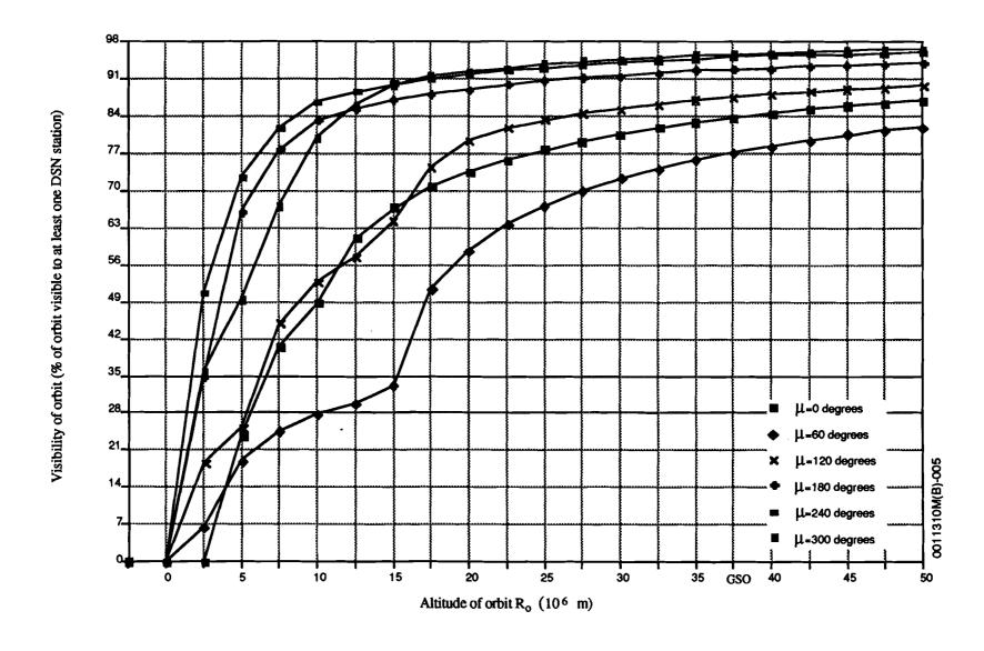
Figure 5. DSN Visibility: As a function of R  $_0$  and  $\mu$  (  $\gamma$  is constant at 28.6 degrees)
