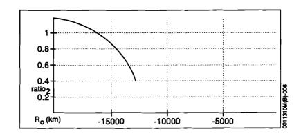
The following graph is a comparison between the visibilities of the simple two-dimensional model and the  $\theta_e$  = 10° elevation angle constraint two-dimensional model (Figure 1 versus Figure 2). The  $\theta_e$  elevation angle constraint plot (ratio') is the dark line on the bottom, indicating the decrease in visibility caused by adding the 10-degree constraint to the LOS.
