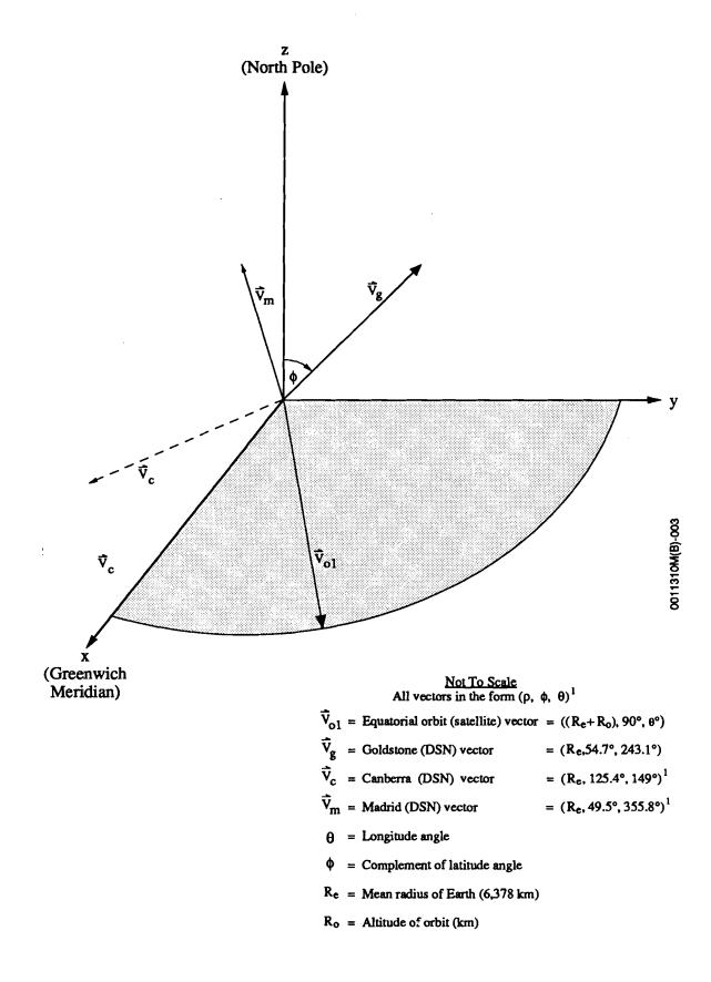
Figure 3. Three-Dimensional Coordinate System
